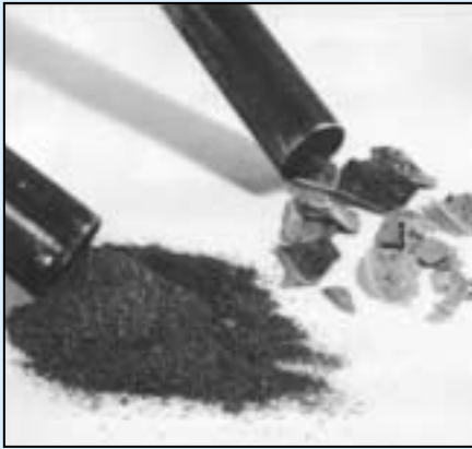
Hard, thick deposits shot from tube after acid cleaning.
