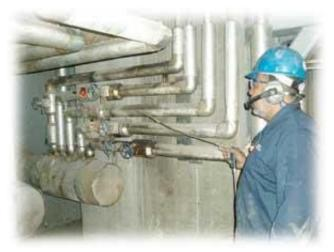
Conco crew supervisor Wayne Holt sprays helium around valves and piping within the vacuum boundary.
