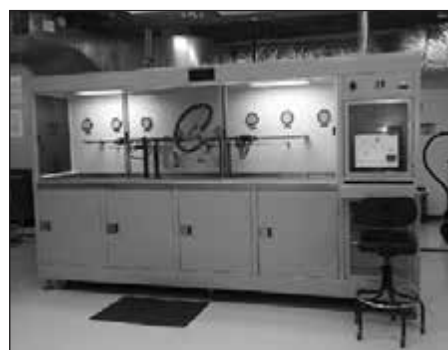
Fluid Care Center: Multi-Pass Test Stand
