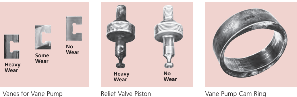
Figure 1. Typical Examples of Wear Due to Contamination
