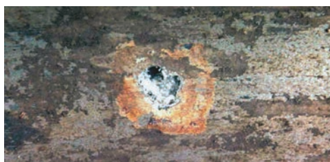
Tube Wall Showing Pitting Due to Magnesium Deposit
