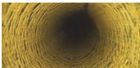
Condenser Tube Fouled with Calcium Carbonate Scale
