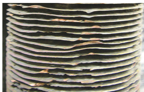
Preheater Fins After Cleaning with NitroLance
