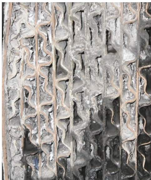
Preheater Basket Before Cleaning with NitroLance
