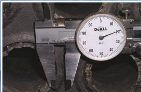
0.320" Thick Hardened Carbon Based Deposit
