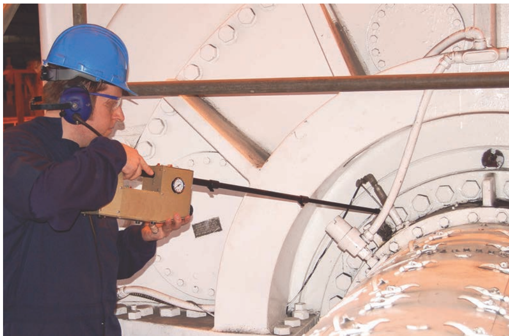
Conco Technician with SF 6 Pack Unit Checking for Sources of Air In-leakage
