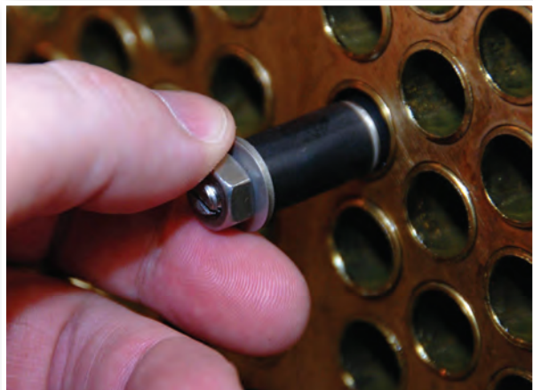
Tube plugging was performed in conjunction with eddy current testing.
