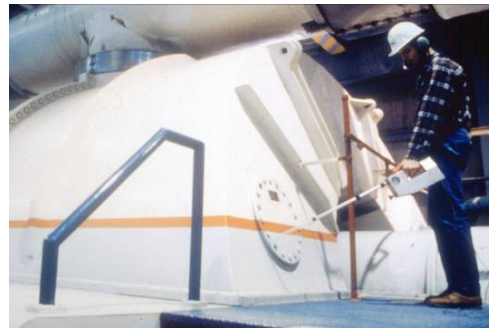
Figure 14 SF6-Pak Hand-held Tracer Gas Dispenser
