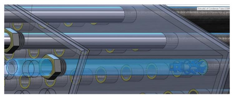
Above is the cleaner coming out of the tube and into the receiver tube shown in a blue tint.
