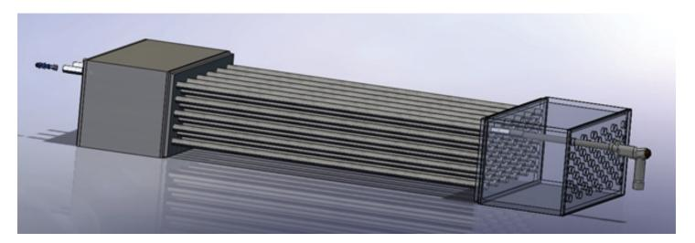
Above you can see that the cleaner and removed deposit (not shown) is carried through the outlet box via the receiver tube and dropped on the other side.
