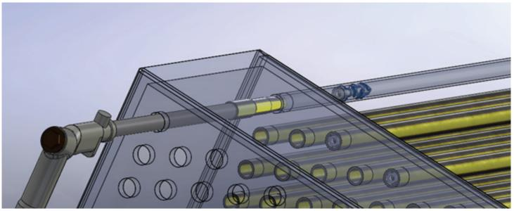
Above is the gun with the extension, shooting water to push the cleaner down the tube and flush deposit.
