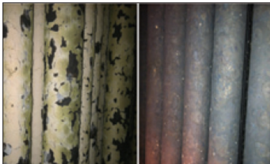
Hot heat exchanger before and after cleaning with NitroLance.™
